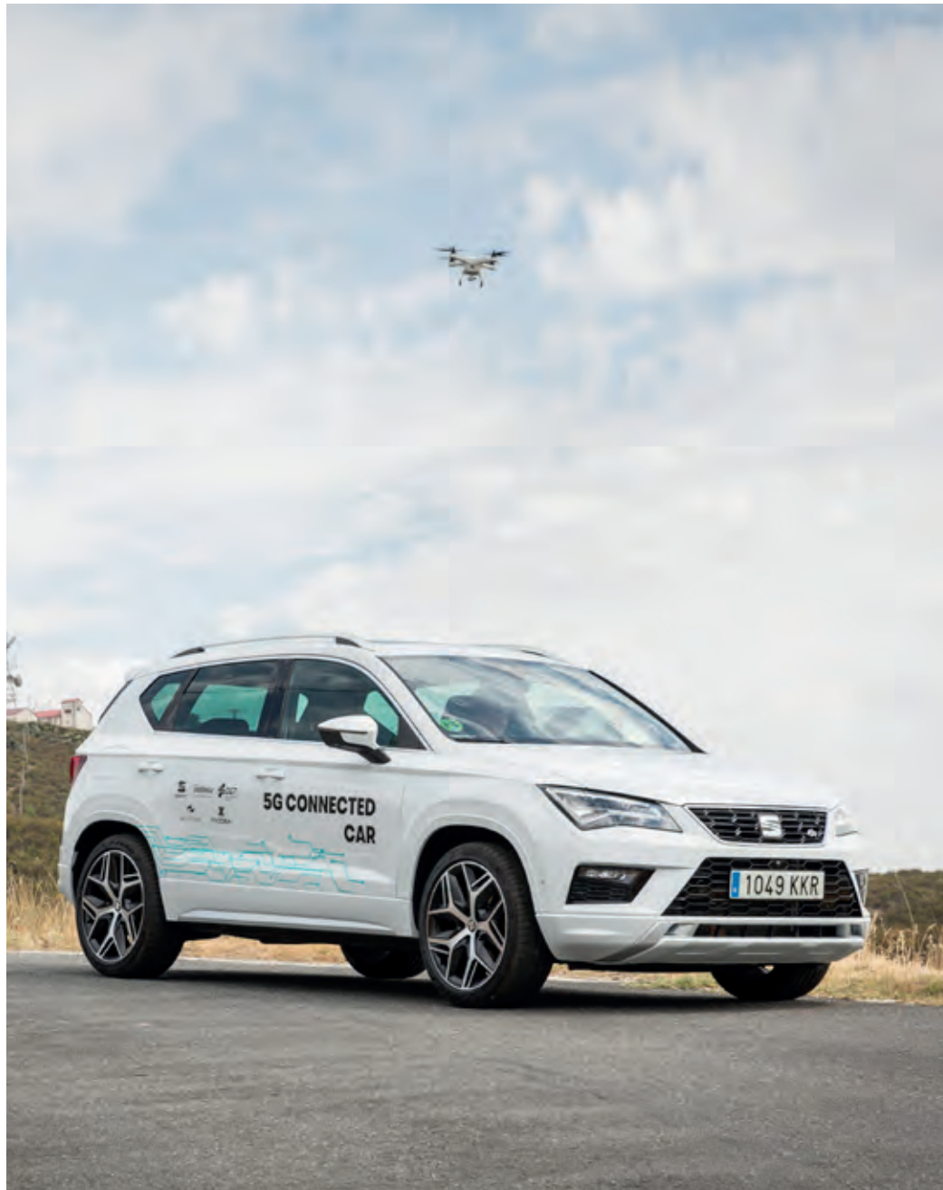
A drone fitted with a camera captures what happens on the road and sends it, via the Telefónica network, to a DGT server.
